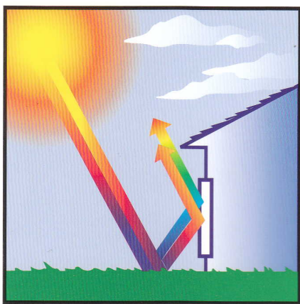
Low-E Glass filters long-wave radiation. This reduces heat gain in your home from the sun in the summer, keeping your home cooler.
